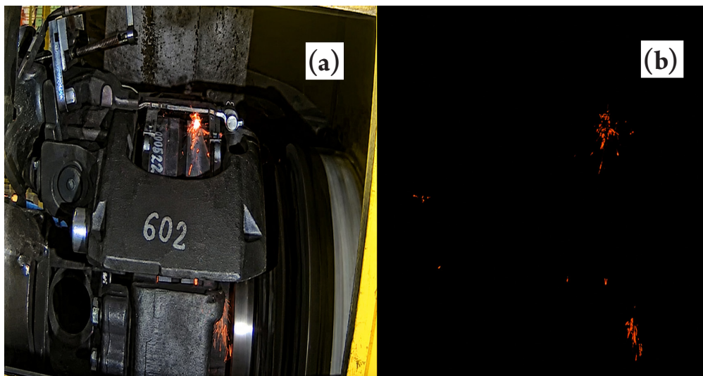
Figure 2. (a) Experimental apparatus used for spark generation and (b) representative image used to evaluate the amount of sparks and flames generated during the FMVSS-121 test procedure.
